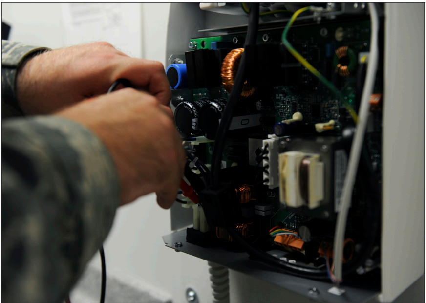
U.S. Air Force Senior Airman Lance Voegtline, a biomedical equipment technician with the 509th Medical Support Squadron, calibrates a dental x-ray power board at Whiteman Air Force Base, Mo., Oct. 13, 2016. The equipment assigned to the medical group are inspected against manufacture, National Fire Protection Association and industry standards.
