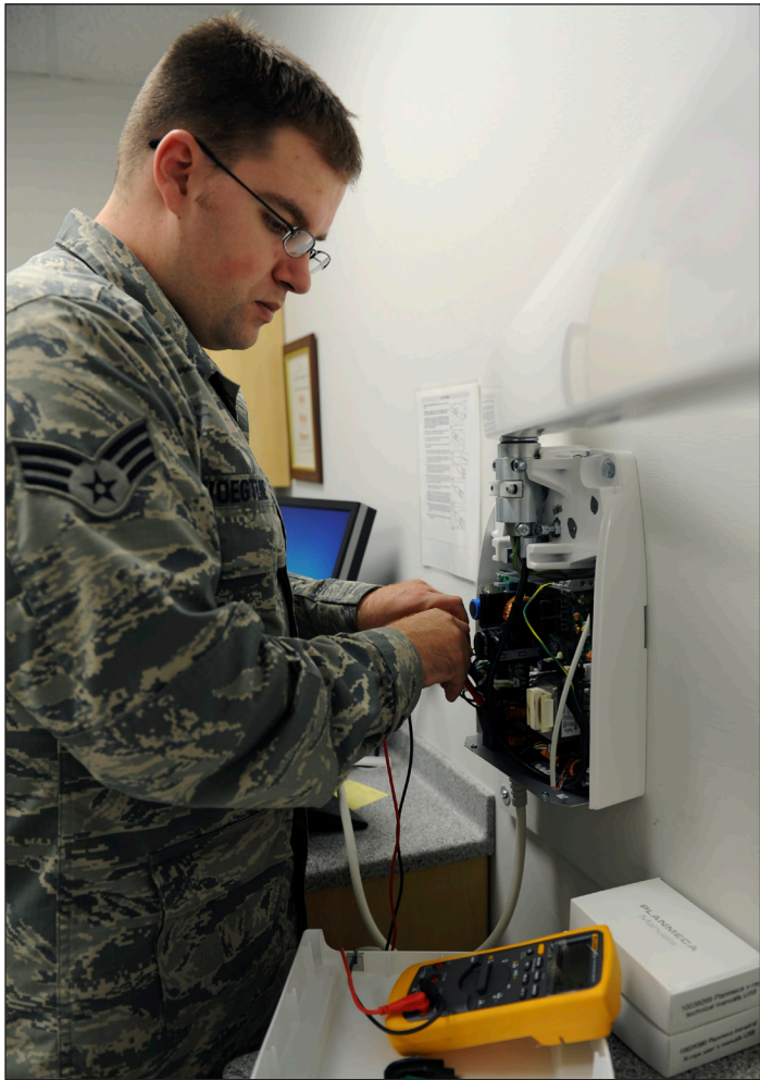
U.S. Air Force Senior Airman Lance Voegtline, a biomedical equipment technician (BMET) with the 509th Medical Support Squadron, inspects a power board for a dental x-ray machine at Whiteman Air Force Base, Mo., Oct. 13, 2016. BMETs stay up-to-date on industry leading equipment and use this knowledge to review and approve all medical equipment that is assigned to the clinic.
