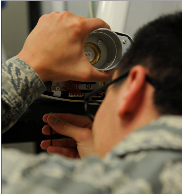
U.S. Air Force Staff Sgt. Pablo Novel-Valdez, a biomedical equipment technician with the 509th Medical Support Squadron, removes the cone from the x-ray tube-head to salvage the parts for later use at Whiteman Air Force Base, Mo., Oct. 11, 2016. Each month Novel-Valdez has a specific list of medical equipment requiring preventive maintenance to ensure they are working efficiently.
